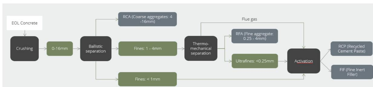
Figure 2. Core C2CA process.
