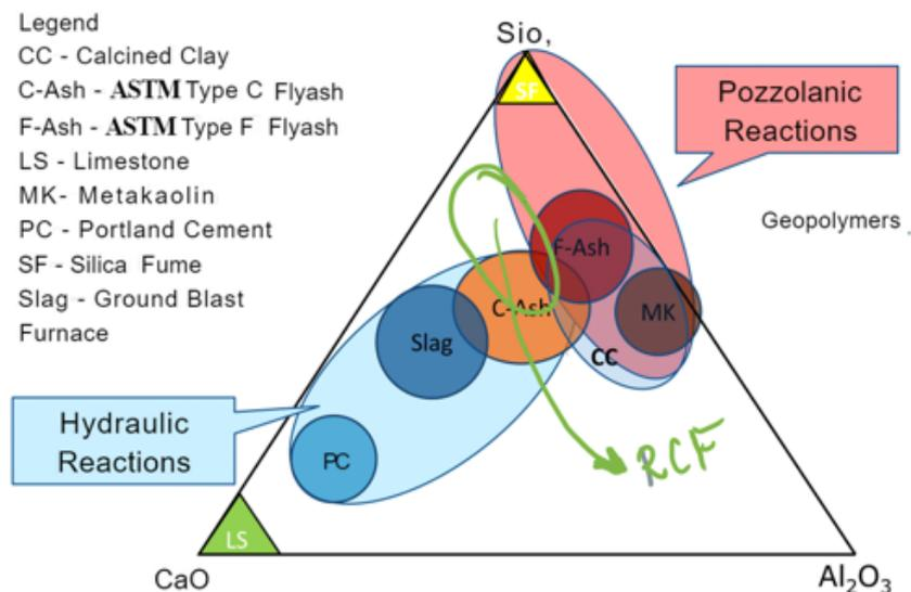
Figure 4. RCF in the Ternary Phase Diagram.
