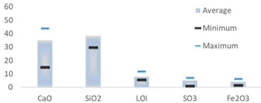
Figure 3. Chemical properties of Recycled Cement Fines (RCF).
